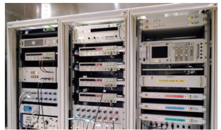
Figure 4 Measurement facility of local calibration service for frequency standards
