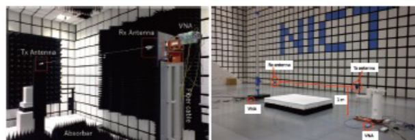
Figure 3 Development of an 18 GHz to 40 GHz antenna calibration method and a validation method for anechoic chamber
