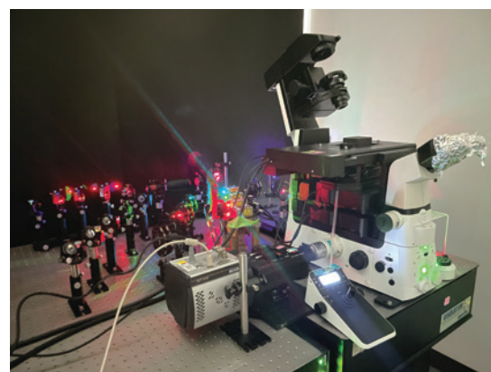
Figure Simultaneous four-color fluorescence microscope system under construction
