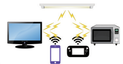
Bad effects of electromagnetic noise to wireless communication
