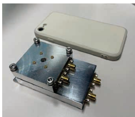
Figure 2 The small charge measurement device currently under development
