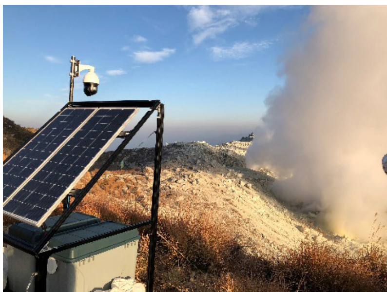
Fig.6 : A field trial of a developed solar-powered sensor for monitoring volcanic activity
