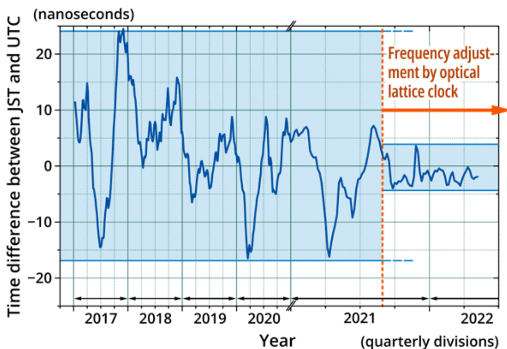
Fig.1 : The difference between Japan Standard Time (JST) and Coordinated Universal Time (UTC) has been reduced from typically \pm 20 ns to less than \pm 5 ns by the inclusion of the optical lattice clock since August 2021.
