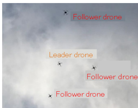
Platooning flight following the leader drone
