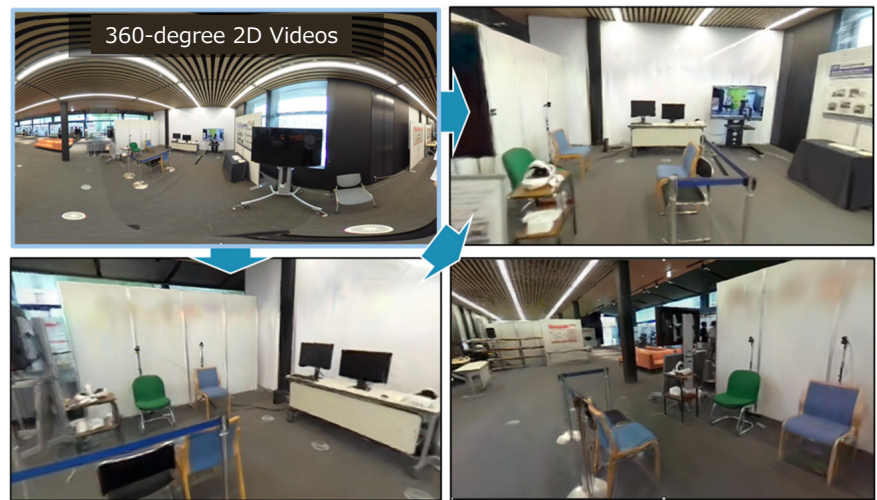
Fig.5 : Constructing 3D digital twins using 360-degree 2D videos and image generation from arbitrary viewpoints
