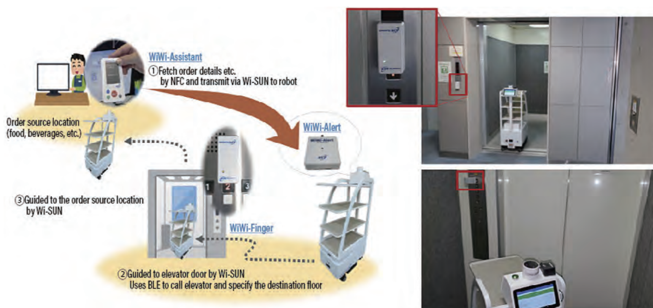
Fig. : Configuration of our experimental multi-story navigation support system using an autonomous mobile delivery robot, and photos of the system in action
