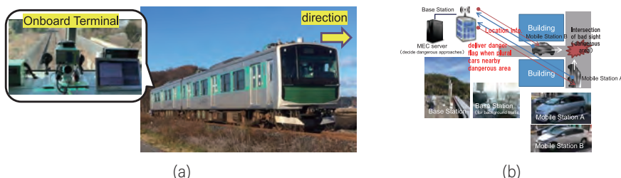
Fig.1 : Wireless network management technology: (a) Railway demonstration experiment employing the private microcell structure, (b) STABLE enhancement verification test harmonized with MEC functions
