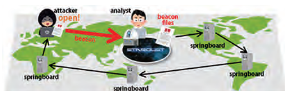
Fig.3 : Concept of medium-scale-attack source attribution using beacon files
