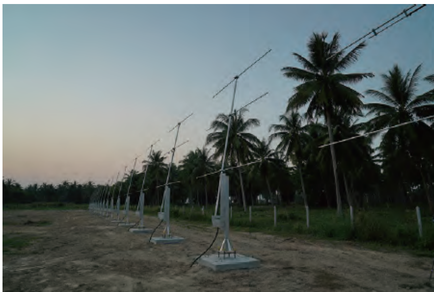
Fig.4 : VHF radar for monitoring Equatorial Plasma Bubbles, installed in Chumphon, Thailand
