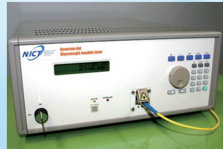
High precision wavelength-tunable quantum dot light source
