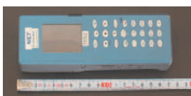
Fig.2: Overview of the Portable Terminal (Weight: 266g; Volume: 264cc; Battery not included)
