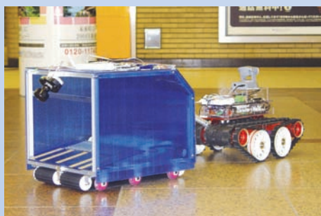
Fig.2: Communication Cable Laying Robot under Joint Development with International Rescue System Institute and Other Research Organizations
