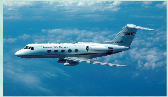
Figure 2: Aircraft Equipped with Pi-SAR2 The antennas are mounted beneath the wings in center of the aircraft.
