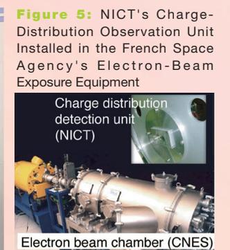
Figure 5: NICT's Charge-Distribution Observation Unit Installed in the French Space Agency's Electron-Beam Exposure Equipment
