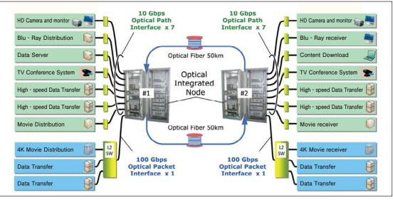
Figure 3 Structure of demonstration network
