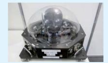
A model of the radio-wave absorbing characteristics of a human head was used to measure interference by radio waves.
