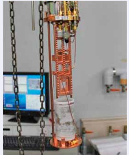
Figure 3 ● Superconducting quantum bit measurement environment in a dilution refrigerator
