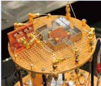
Figure 2 ● SFQ circuits mounted in an ultra-low temperature refrigerator
