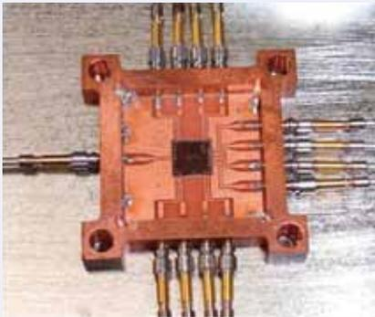
Figure 1 ● Small block for mounting SFQ circuits
