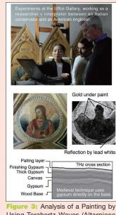
Figure 3: Analysis of a Painting by Using Terahertz Waves (Altarpiece by Giotto, Tempera Painting, around 1300 A.D.)
