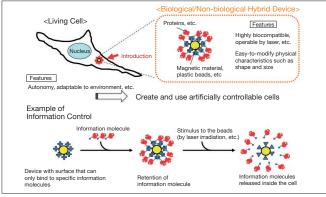
Figure 2: Creating Cells with Embedded Biological/Non-biological Hybrid Devices
