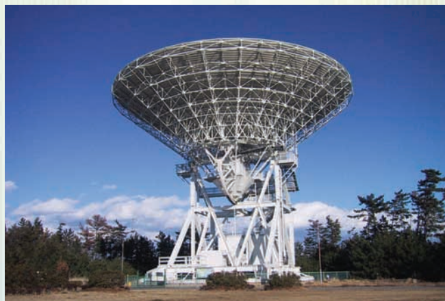
Fig.3: Radio Telescope Used for VLBI Observation (Kashima Space Research Center)
