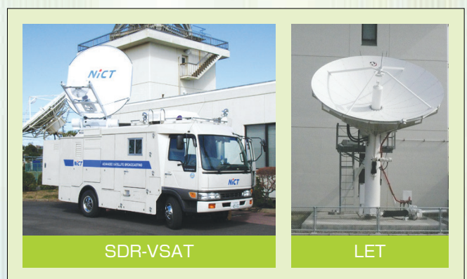
Fig.4: Large Earth Terminal and Super-High Data-Rate Very Small Aperture Terminal
