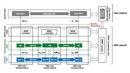
Figure 2 Basic configurations of the QKD network and user network specified in the international standard recommendation, ITU-T Y.3800
