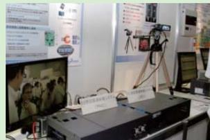
The Ultra High-speed Image Transmission Technology using Millimeter Wave successfully transmits an uncompressed full high-definition video without delay.
