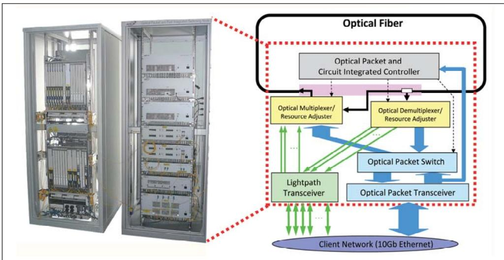
Figure 2 ● Developed optical packet and circuit integrated node
