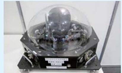
A model of the radio-wave absorbing characteristics of a human head was used to measure interference by radio waves.
