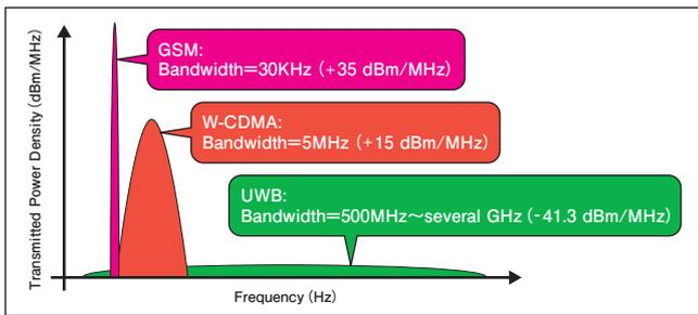
Figure 3 ● Power spectrum of UWB and narrowband signal
