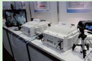
The Broadband Mobile Communication System for Public Safety allows fire-fighters and policemen to transfer high-definition video of the disaster-stricken site to the task force in real time.
