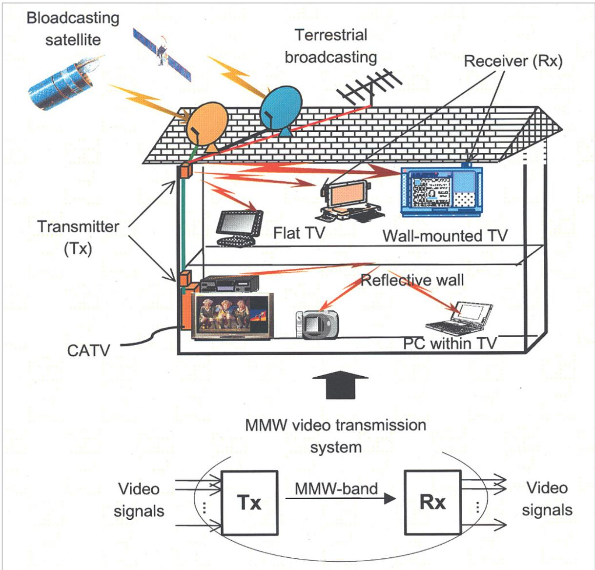
**Fig. 1** Conceptual image of MMW video transmission system
