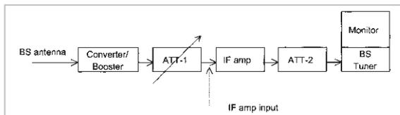
**Fig. 15** Experimental setup for evaluating IM3 products
