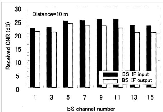
**Fig. 19** Experimental CNR before and after MMW transmission
