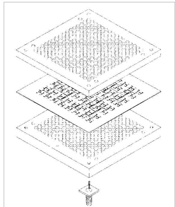
**Fig. 11** Schematic structure of  $16 \times 16$  array antenna
