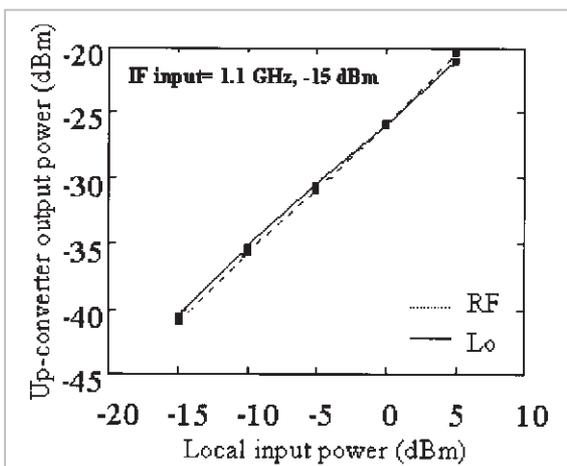
**Fig.5** Local input power vs. up-converter output power
