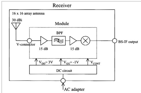
**Fig. 8** Block diagram of receiver
