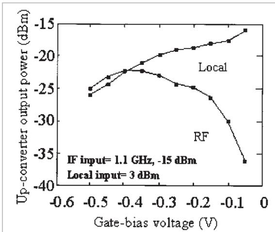
**Fig.4** Gate-bias voltage vs. up-converter output power applied in the balanced mixer
