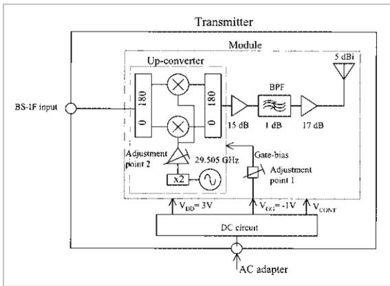
**Fig.3** Block diagram of transmitter
