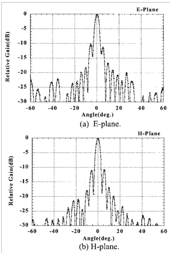
**Fig. 13** Far field pattern of 16X16 array antenna
