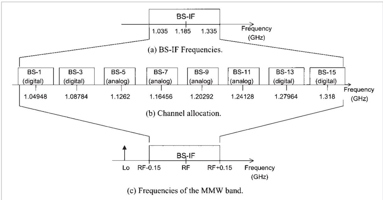
**Fig.2** BS-IF frequencies, channel allocation, and frequencies of MMW band
