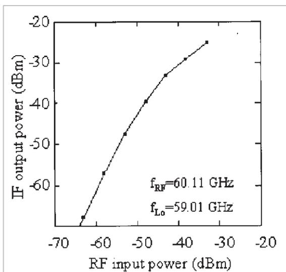
**Fig. 10** RF input power vs. IF output power of receiver
