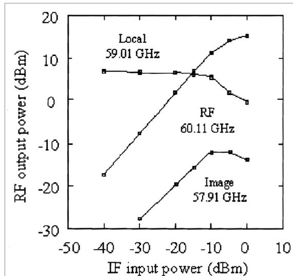
**Fig.7** IF input power vs. RF output power of transmitter
