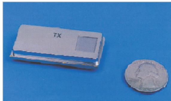
**Fig.6** RF module in transmitter
