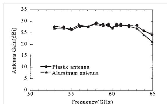
**Fig. 14** Antenna gain of plastic-base and of aluminum-base antennas
