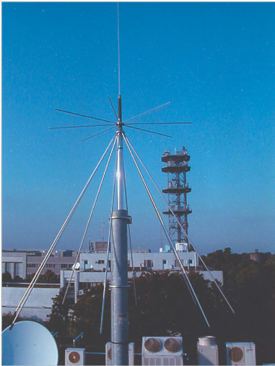
Fig. 9 Discone antenna for use in the present experiment
