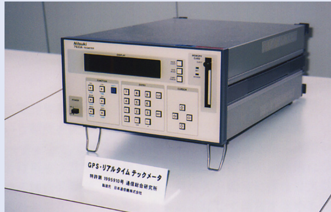
External view of the GPS Real-Time TECMETER (Total Electron Content Meter)
