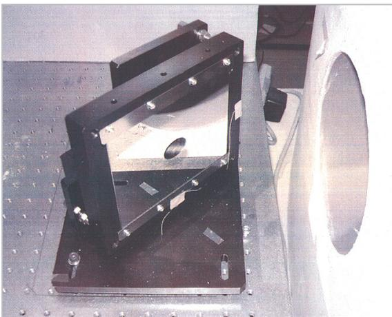
**Fig.3** Center-bored mirror that connects the light-sending and -receiving systems (single column)
