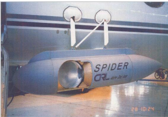
**Fig.2** Radar pod with antenna exposed
