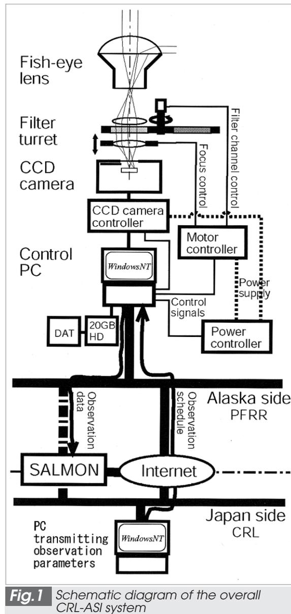
**Fig.1** Schematic diagram of the overall CRL-ASI system
