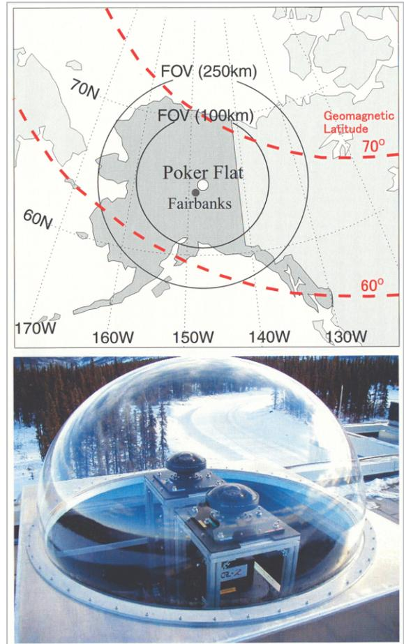
**Fig.4** Observation field of view and the state of installation of the CRL imagers
