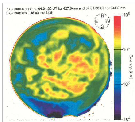
**Fig.8** A horizontal distribution of average energies of precipitating electrons estimated from ratios of illuminance at 427.8 nm to that at 844.6 nm
