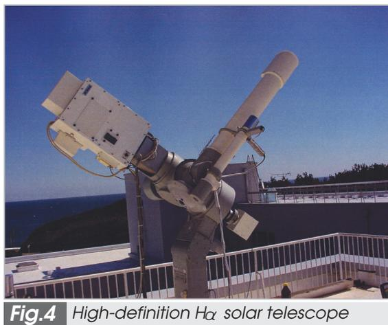
**Fig.4** High-definition  $H\alpha$  solar telescope
