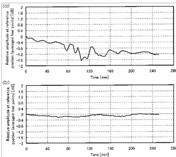
**Fig.6** Amplitude characteristic curve of reference signal power (40 GHz). (a) Measurement 1, (b) Measurement 2
