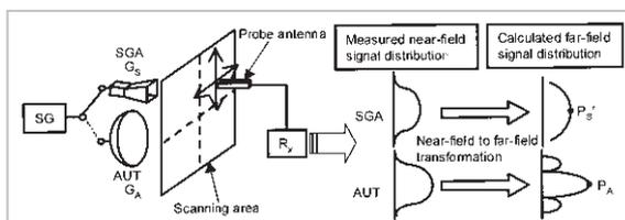
**Fig.2** Antenna gain measurement using the gain-transfer method (near-field antenna measurement)
