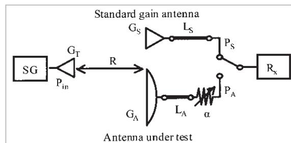
**Fig. 1** Antenna gain measurement using the gain-transfer method (far-field antenna measurement)
