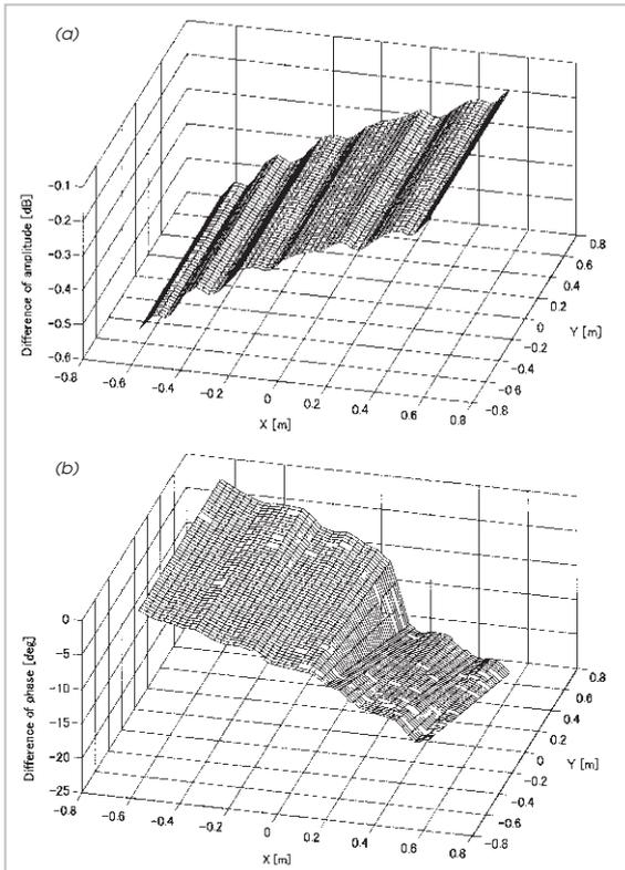
**Fig.9** Difference in near-field distribution before and after correction using the reference signal power curve (at 28 GHz, in Measurement 1). (a) Difference in amplitude distribution (b) Difference in phase distribution
