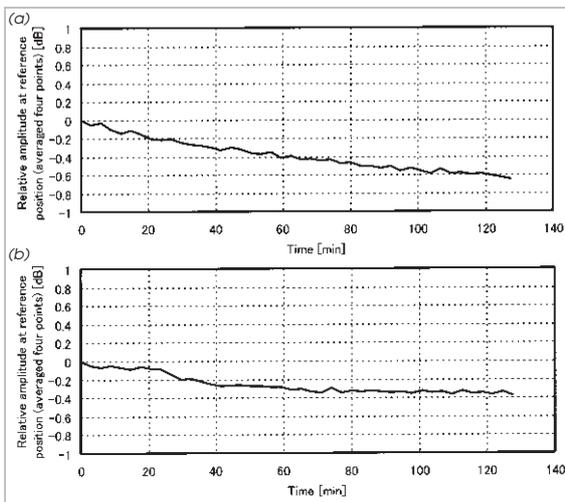
**Fig.5** Amplitude characteristic curve of reference signal power (28 GHz). (a) Measurement 1, (b) Measurement 2
