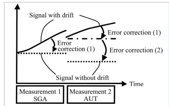
**Fig.3** Schematic diagram of signal drift in measurement of antenna gain employing the near-field antenna measurement
