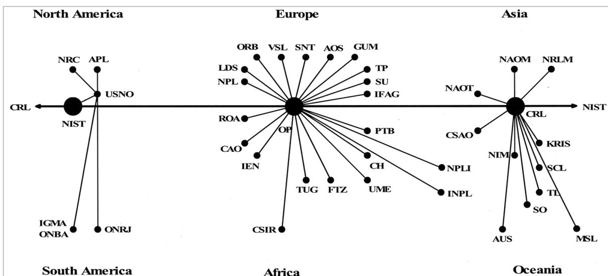
**Fig. 1** International time transfer network contributing to TAI as of the beginning of the 1990s (Only the single-frequency, single-channel GPS common-view method is used in comparison.)
