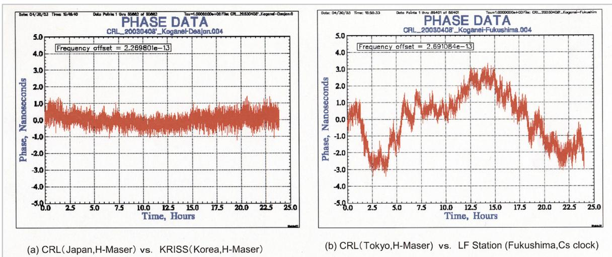
**Fig.5** Results of time/frequency transfer among three stations (CRL Koganei, Korea's KRISS, and the CRL Mt. Ohtakadoya LF Station) using multi-channel two-way satellite time/frequency transfer modem
