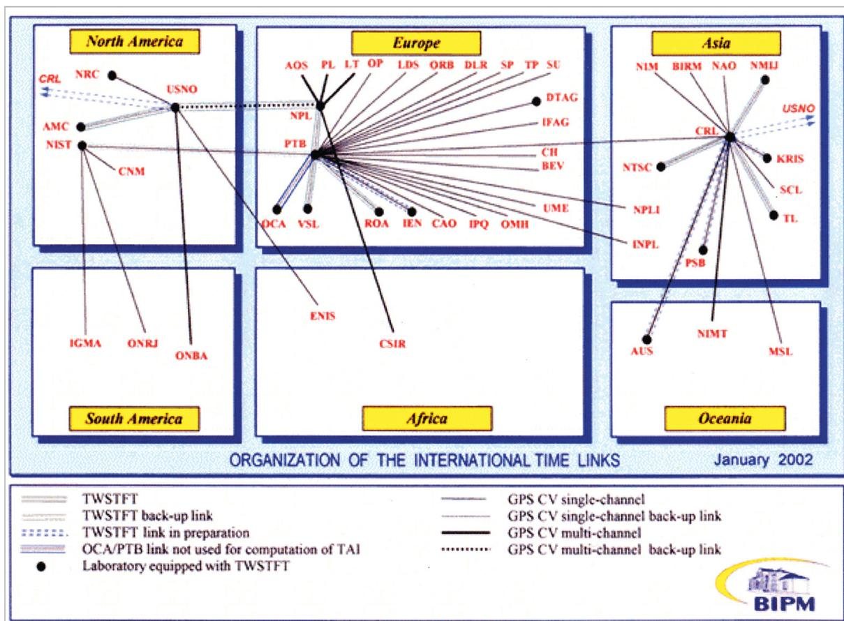
**Fig.2** International time links for the calculation of TAI, as of January 2002 (From the BIPM website. The single-frequency single-channel GPS Common-view method, the multi-channel version of this method, and two-way satellite time and frequency transfer are combined to form a unified system of time comparison.)
