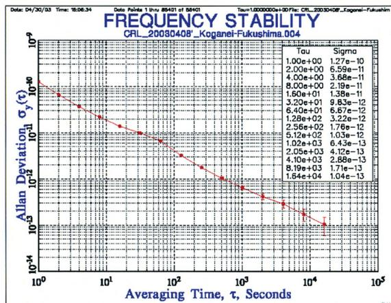
(b) CRL(Tokyo,H-Maser) vs. LF Station (Fukushima,Cs clock)
