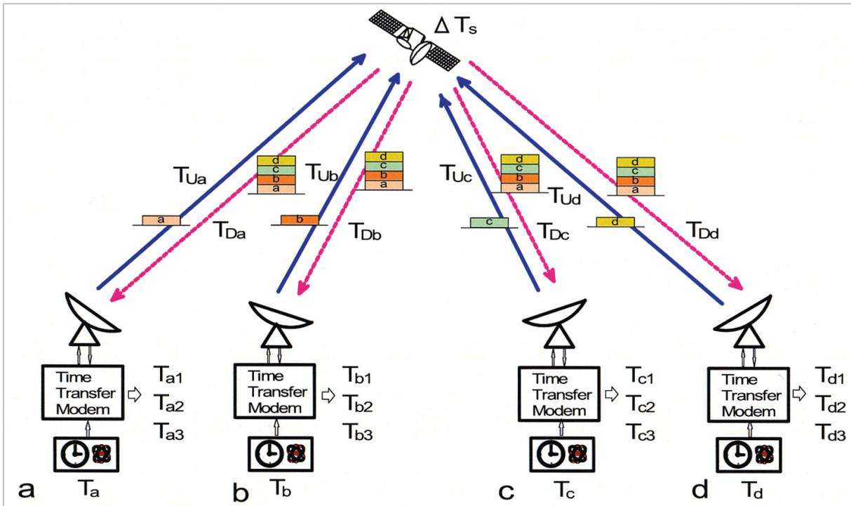
**Fig.3** Conceptual diagram of multi-site simultaneous time transfer using multi-channel two-way satellite time/frequency transfer modem
