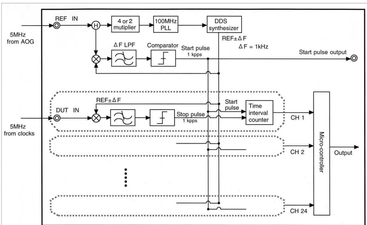
**Fig.5** Block diagram of DMTD system
