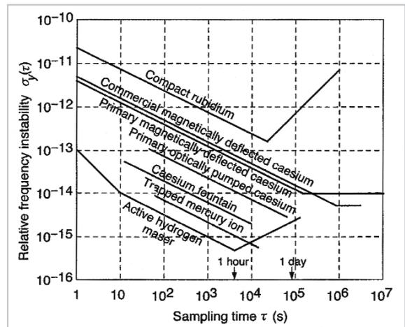
**Fig.4** The frequency stability of various atomic clocks
