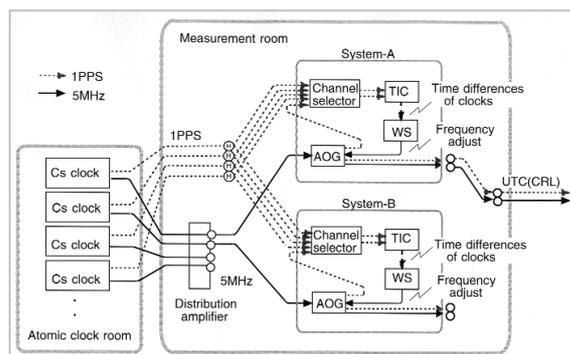
**Fig.2** Current system for generating and measurement of JST (4th generation). TIC: Time interval counter, WS: Workstation
