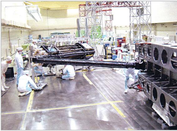
**Fig. 10** Boom deployment test
