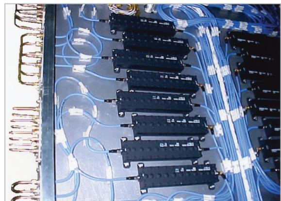
**Fig.4** Filter arrangement in Rx unit
