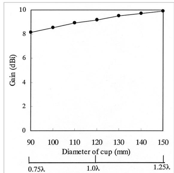
**Fig.3** Element gain vs. cup diameter. (cup height = 50 mm)
