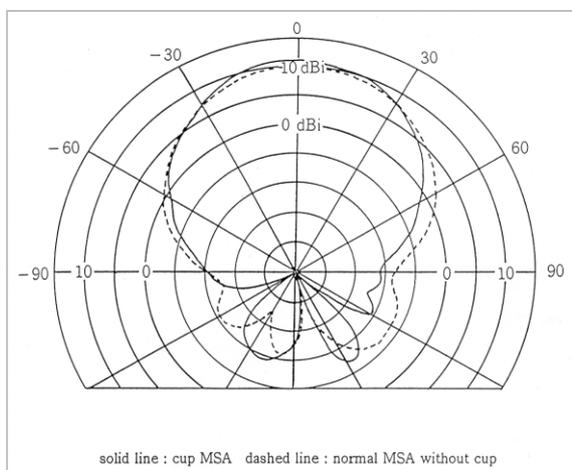
**Fig.4** Element pattern of a cup MSA compared with that of a normal MSA.
