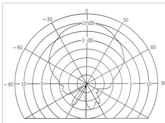
**Fig.5** Element pattern of a cup MSA in an array. (element spacing =  $1\lambda$ )
