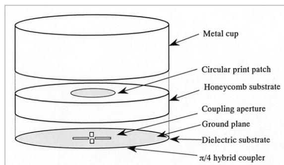
**Fig. 1** Structure of a honeycomb-based cup MSA.
