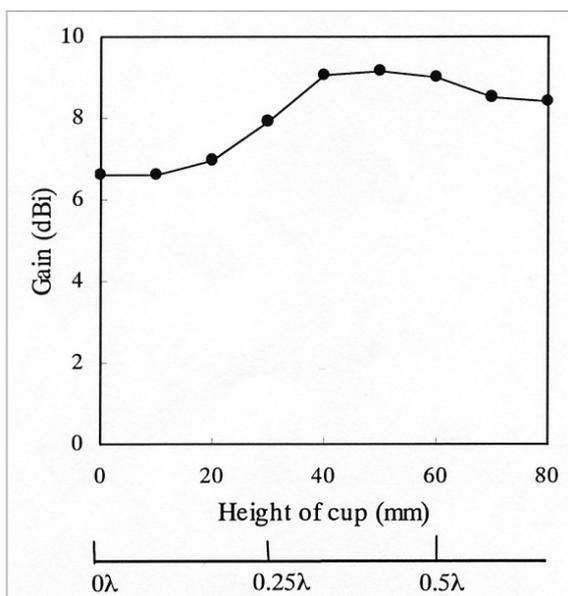
**Fig.2** Element gain vs. cup height. (cup diameter =  $1\lambda$ )
