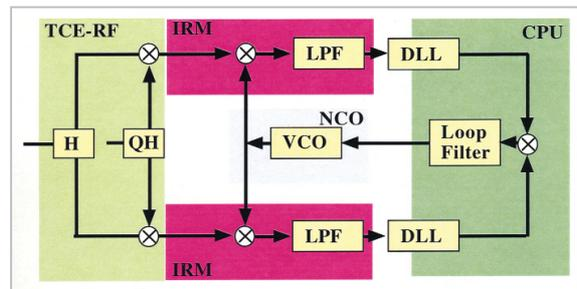
Fig.6 Signal processing system block diagram
