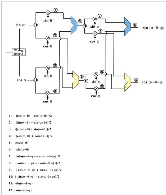
**Fig.2** Principle of IRM D/C
