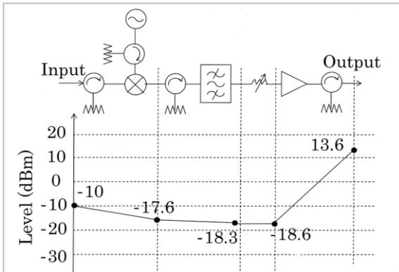
**Fig.3** Diagram of power levels at consecutive stages of up converter
