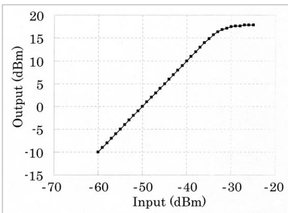
**Fig.7** Input/output characteristics of the LNA at 2502.2 MHz
