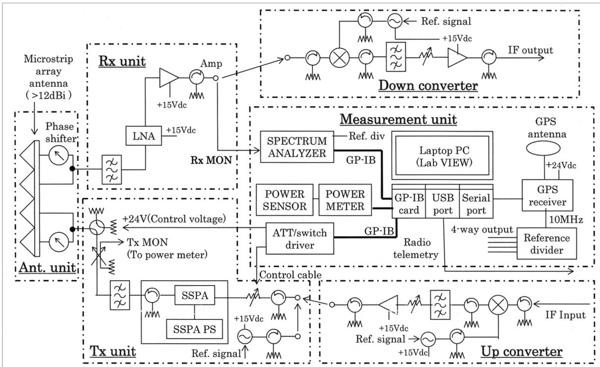
**Fig. 1** Block diagram of the portable earth station
