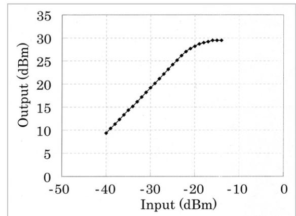
**Fig. 9** Input/output characteristics of amplifier in the down converter at 140 MHz
