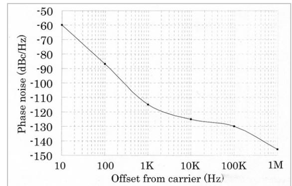
**Fig.10** Phase noise of the local oscillator in the down converter at 2363.5 MHz
