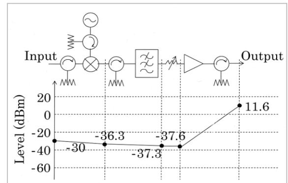
**Fig.8** Diagram of power levels at consecutive stages of down converter
