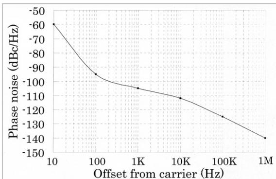
**Fig.4** Phase noise of the local oscillator in the up converter at 2517.5 MHz
