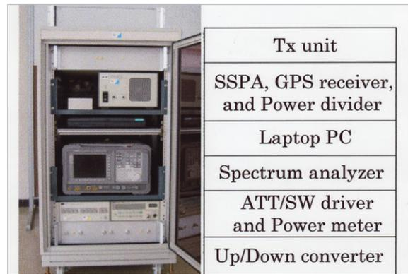
**Fig.2** Appearance and configuration diagram of the portable earth station prototype ((a) photograph of the portable earth station; (b) configuration diagram)
