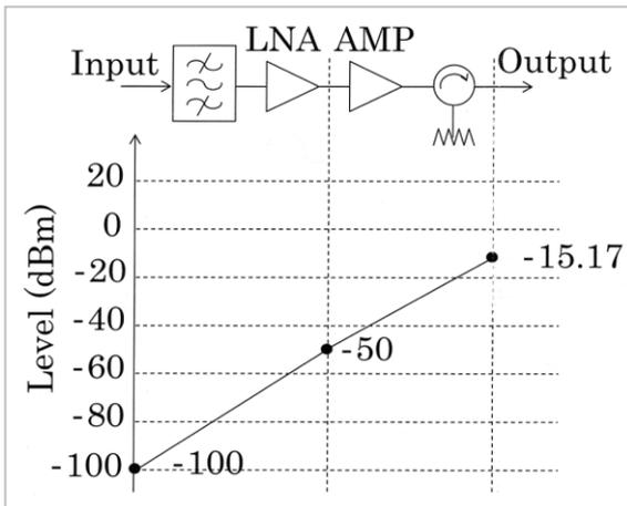
**Fig. 6** Diagram of power levels at consecutive stages of receiving unit
