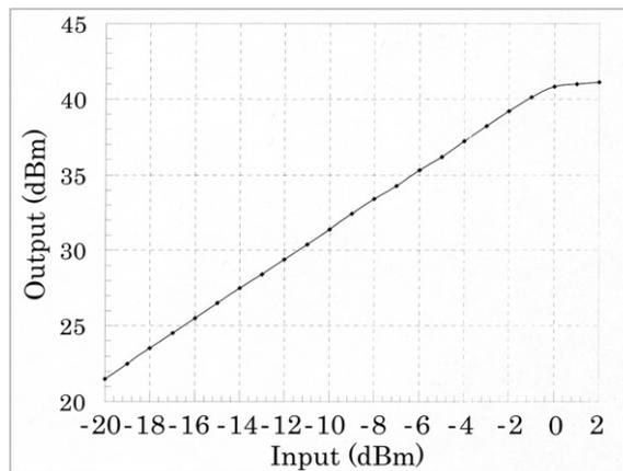
**Fig.5** Input/output characteristics of the transmission unit at 2657.5 MHz
