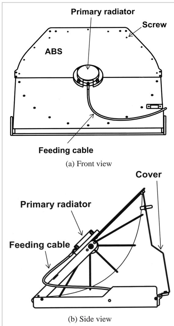
**Fig.4** Structure of the deployed prototype antenna
