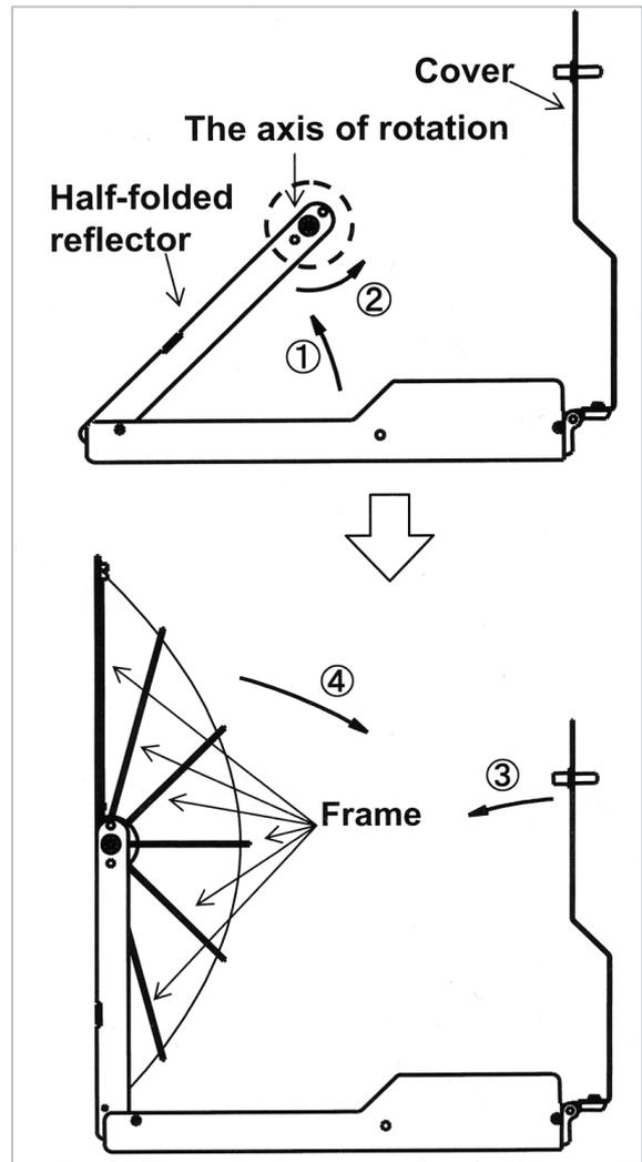
**Fig. 3** Deployment mechanism of the prototype parabolic reflector antenna (side view)
