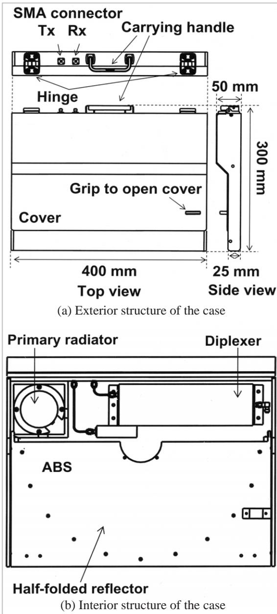
**Fig. 2** Exterior appearance and interior structure of the prototype antenna
