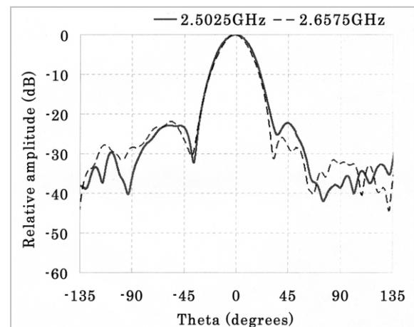
**Fig.6** Radiation patterns of the prototype parabolic antenna
