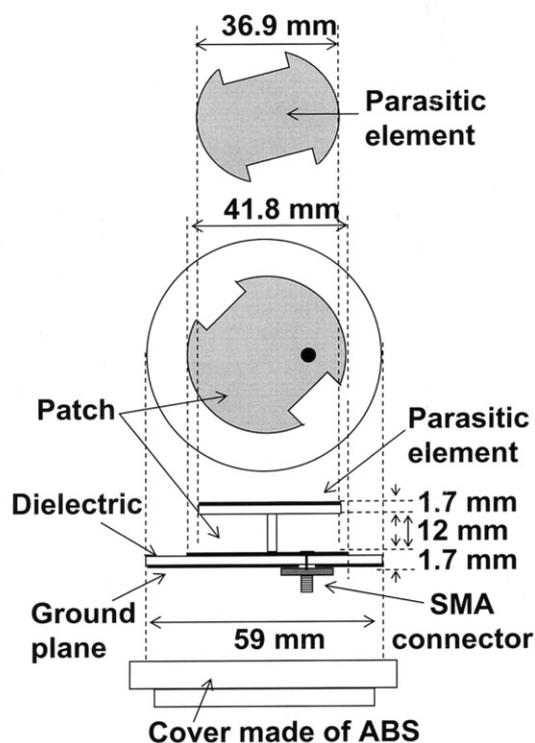
(b) Schematic diagram of the primary radiator
