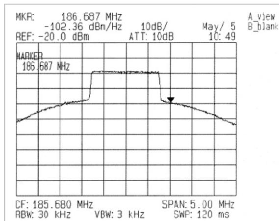
**Fig. 12** SEM output spectrum (IBO = 0 dB)
