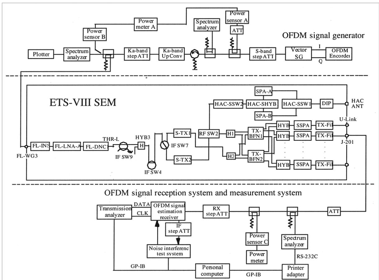
**Fig.9** An example of an SEM test system diagram
