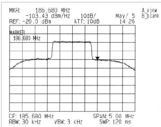
**Fig. 14** SEM output spectrum (IBO = -6 dB)
