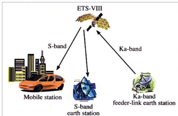
Fig.1 Overview of satellite audio broadcasting experiments
