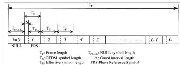
**Fig.4** Composition of transmission frame
