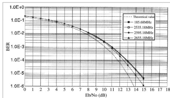
**Fig.8** Loop back BER characteristics in S-band (before error correction)
