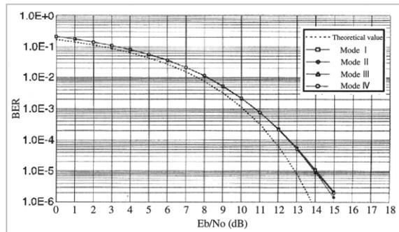
**Fig.7** Loop back BER characteristics in IF (before error correction)
