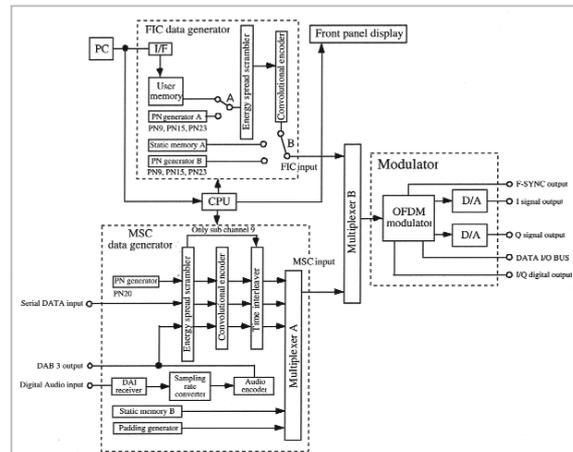
**Fig.3** Block diagram of OFDM signal generator
