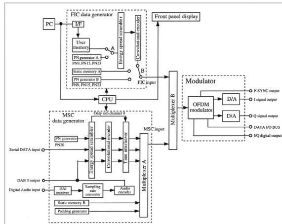
Fig.3 Block diagram of OFDM signal generator
