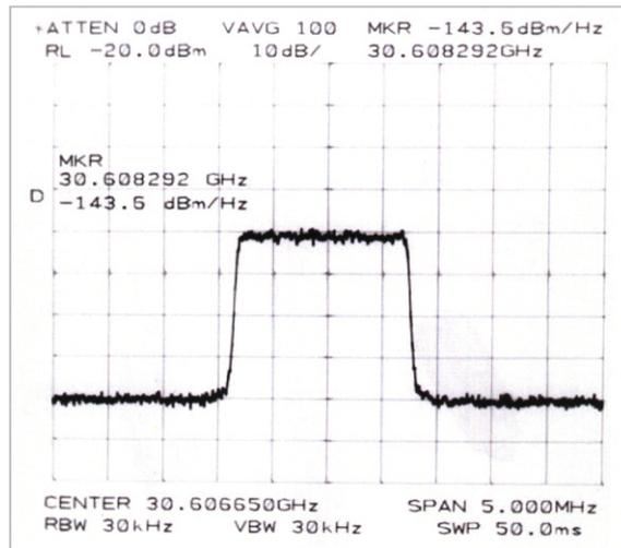
**Fig. 11** Output spectrum of Ka-band up-converter
