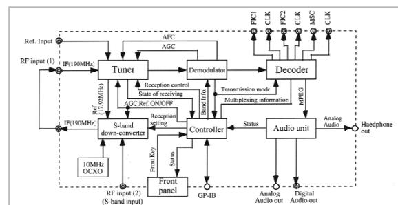
**Fig.6** Block diagram of OFDM signal estimation receiver
