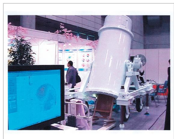
**Fig. 1** Mobile SQUID system in operation at Makuhari Messe convention center
