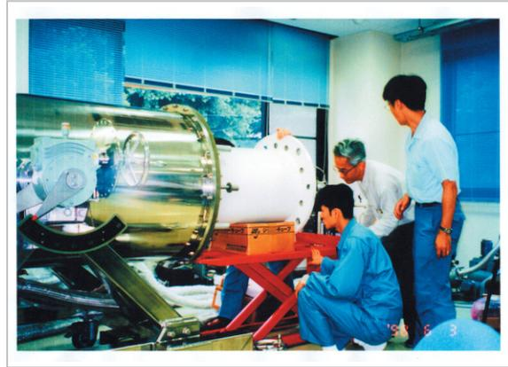
**Fig.4** The SQUID dewar is inserted horizontally.
