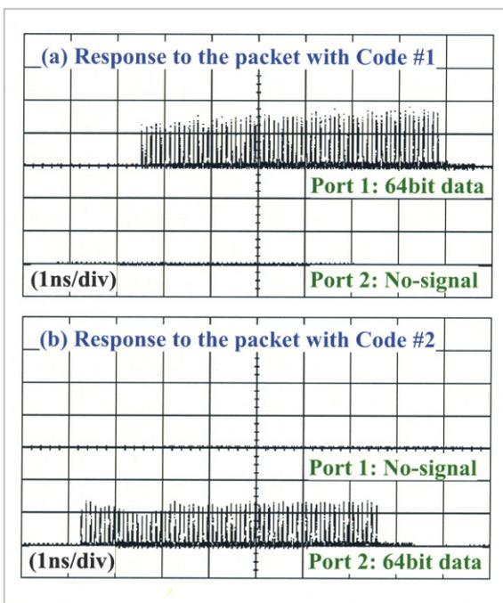
**Fig.6** Routed packet data with code (a) #1 and (b) #2
