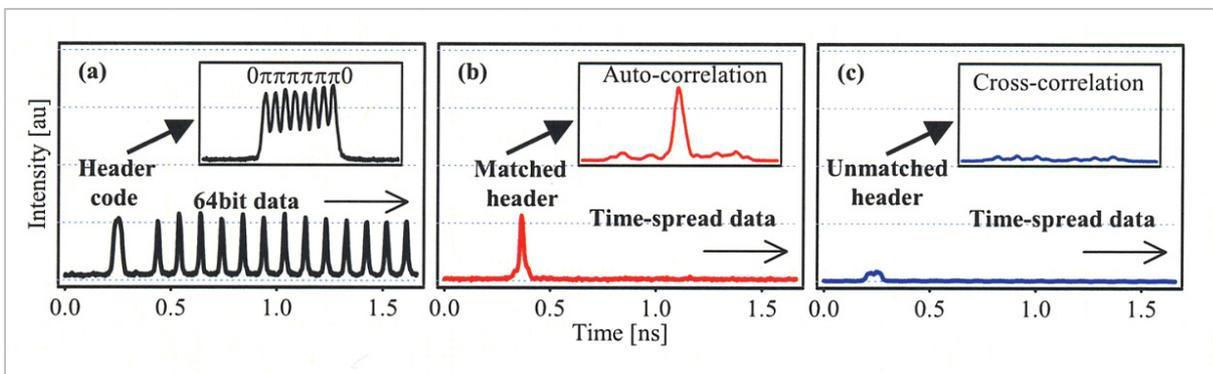
**Fig.5** Streak camera trace of (a) generated packet and correlated signals in (b) matched and (c) unmatched cases
