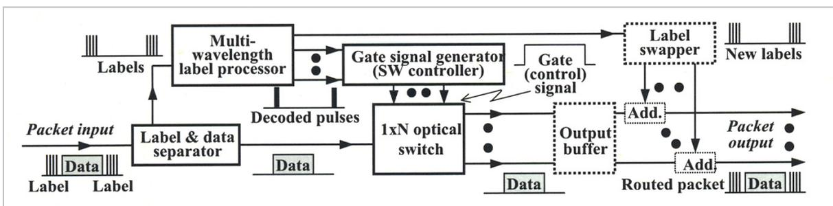
**Fig.9** Multi-wavelength label switch node for variable length packet
