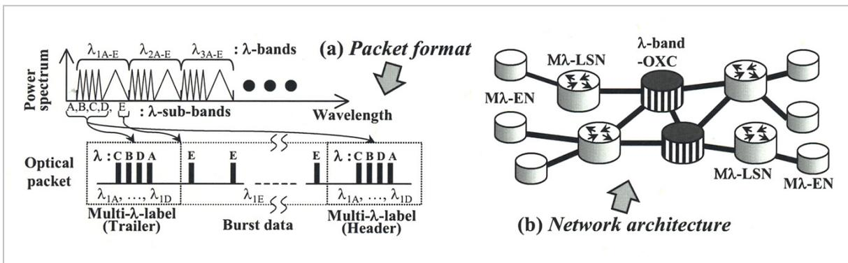
**Fig.8** (a) Packet format and (b) network architecture
