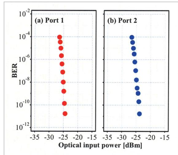
**Fig.7** Measured BER at (a) Port 1 and (b) Port 2
