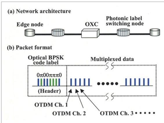
**Fig.2** (a) Network architecture and (b) packet format
