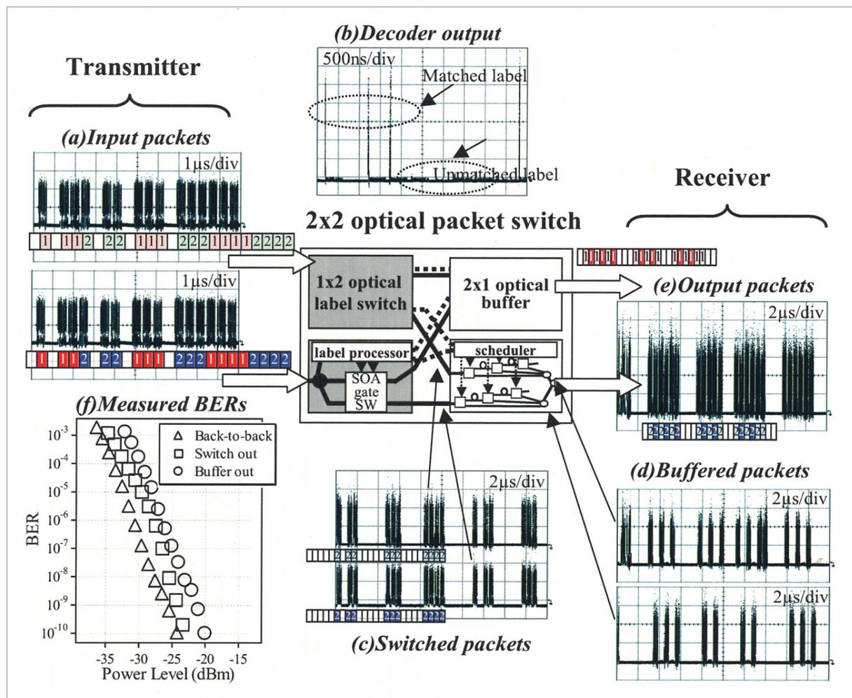
**Fig. 14** Experimental demonstration of OPS prototype
