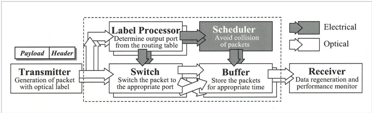
**Fig. 13** Block diagram of the prototype
