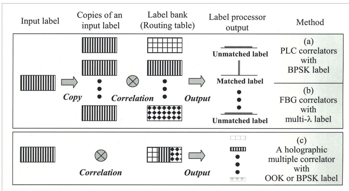
**Fig. 1** All-optical label processing methods
