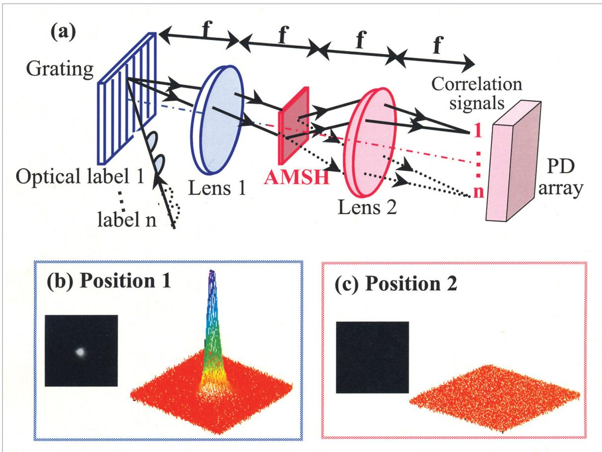
**Fig. 12** (a) Holographic label processor and measured intensity distribution at (b) Position 1 and (c) Position 2
