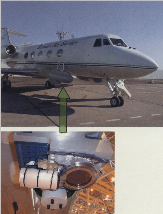
**Fig.2** Airborne coherent Doppler lidar
