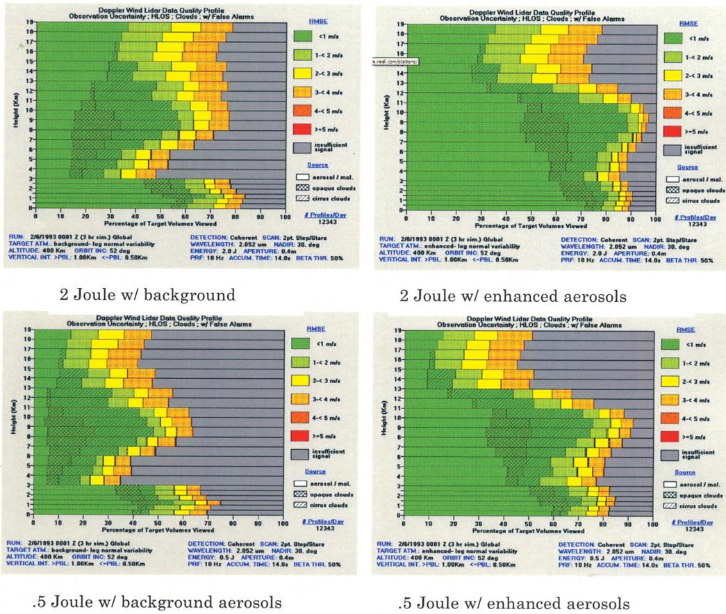
**Fig.8** Doppler wind lidar data quality profiles simulated for JEM/CDL (upper figures) and reduced energy model (lower figures)
