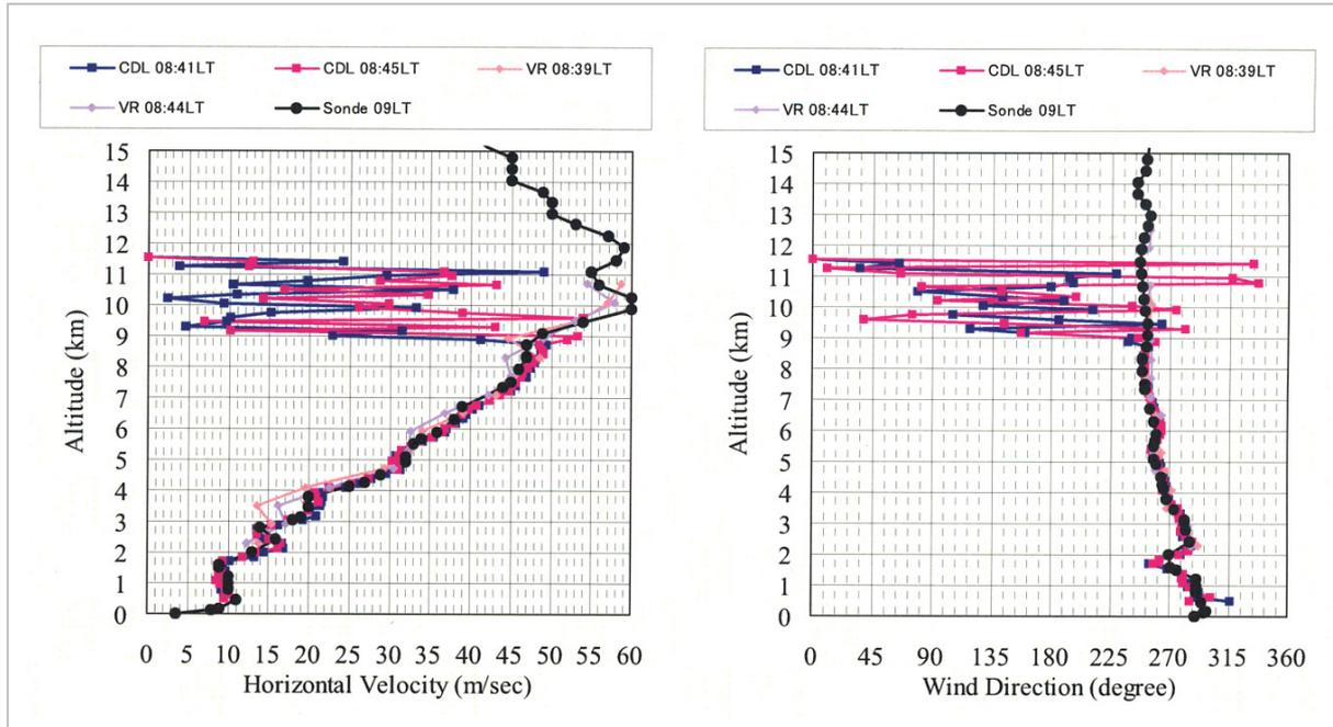
**Fig.5** Wind velocity and direction observed by coherent Doppler lidar(CDL), VHF radar(VR), and radio sonde (Sonde)
