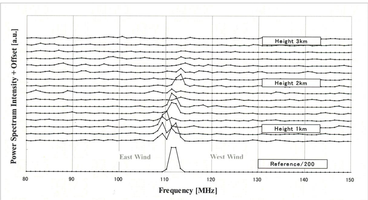
**Fig.4** Spectrum intensities derived from one shot data
