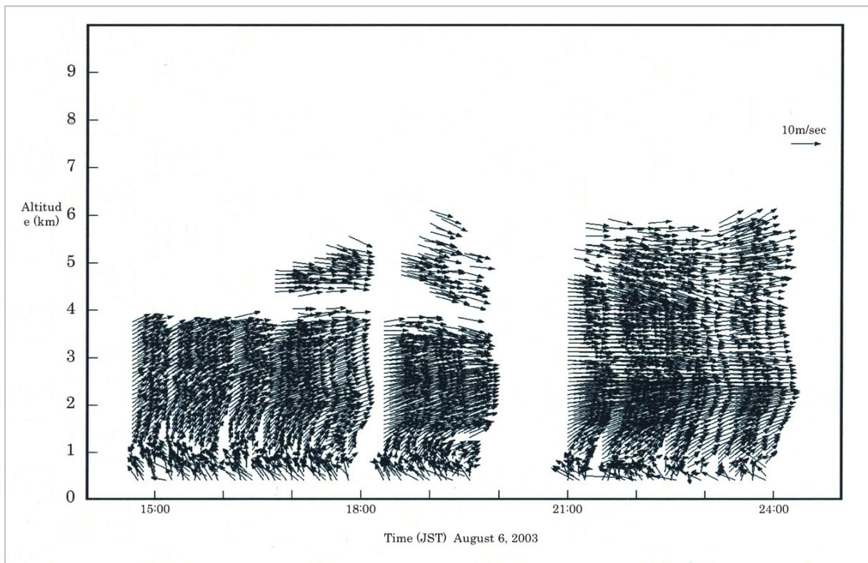
**Fig.6** Time series of wind profiles observed near Kiyokawa on August 8, 2003
