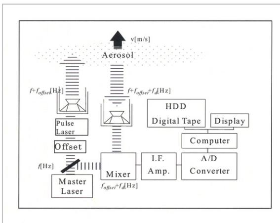
**Fig. 1** Schematic of Coherent Doppler lidar
