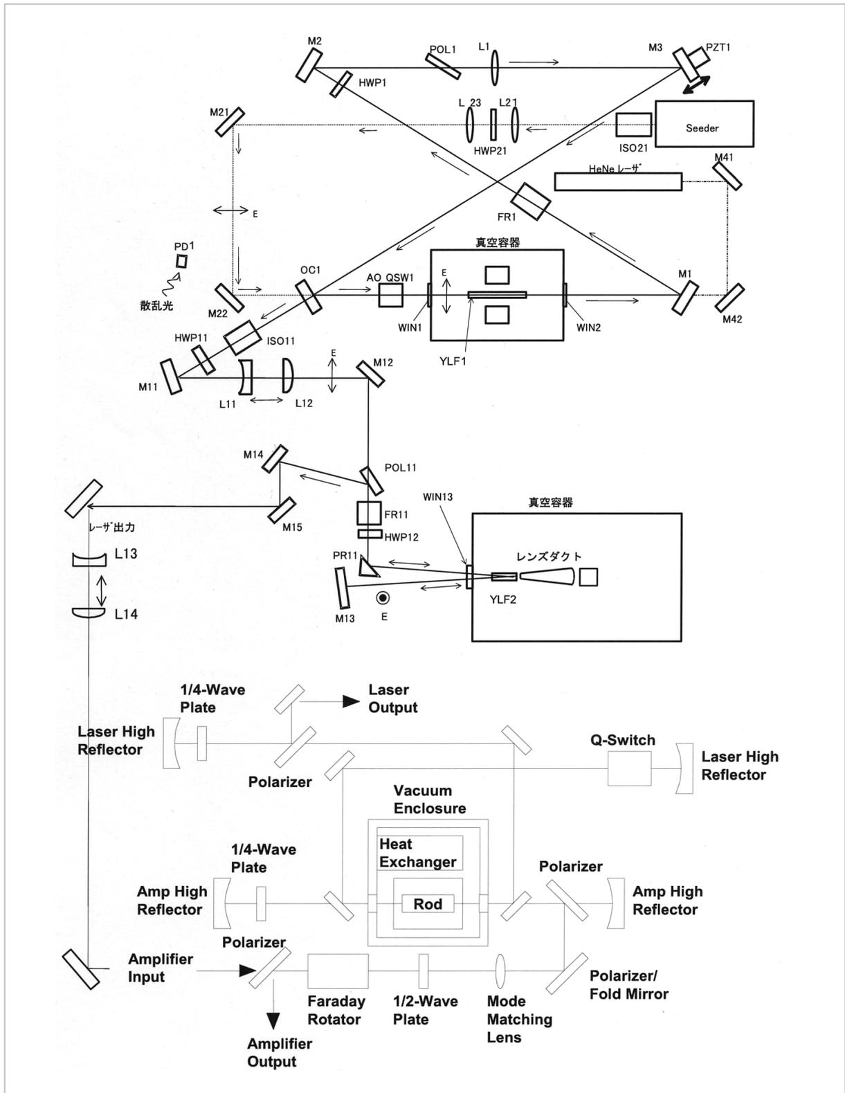
**Fig.9** Layout of the sub-scale laser
