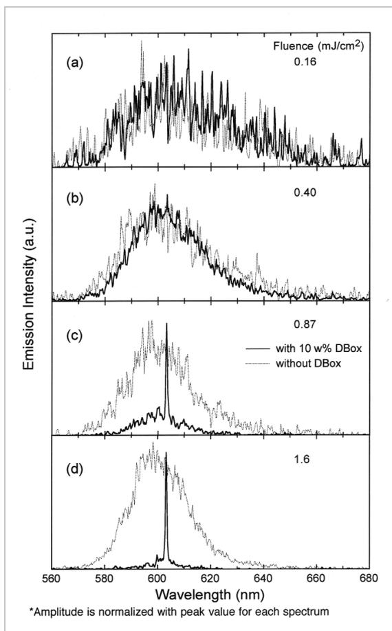
**Fig.6** Laser oscillation spectra of dendrimer/PMMA thin film
