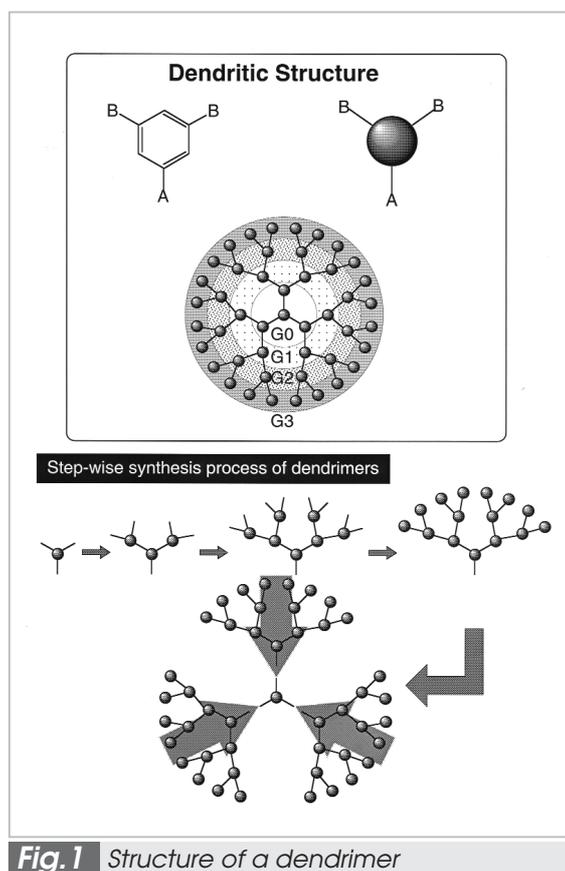
**Fig. 1** Structure of a dendrimer
