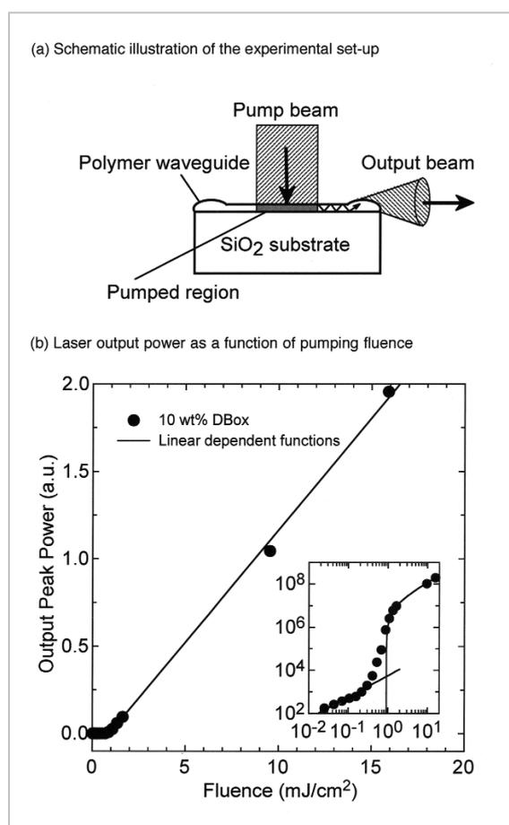
**Fig.5** Laser output characteristics of dendrimer/PMMA thin film
