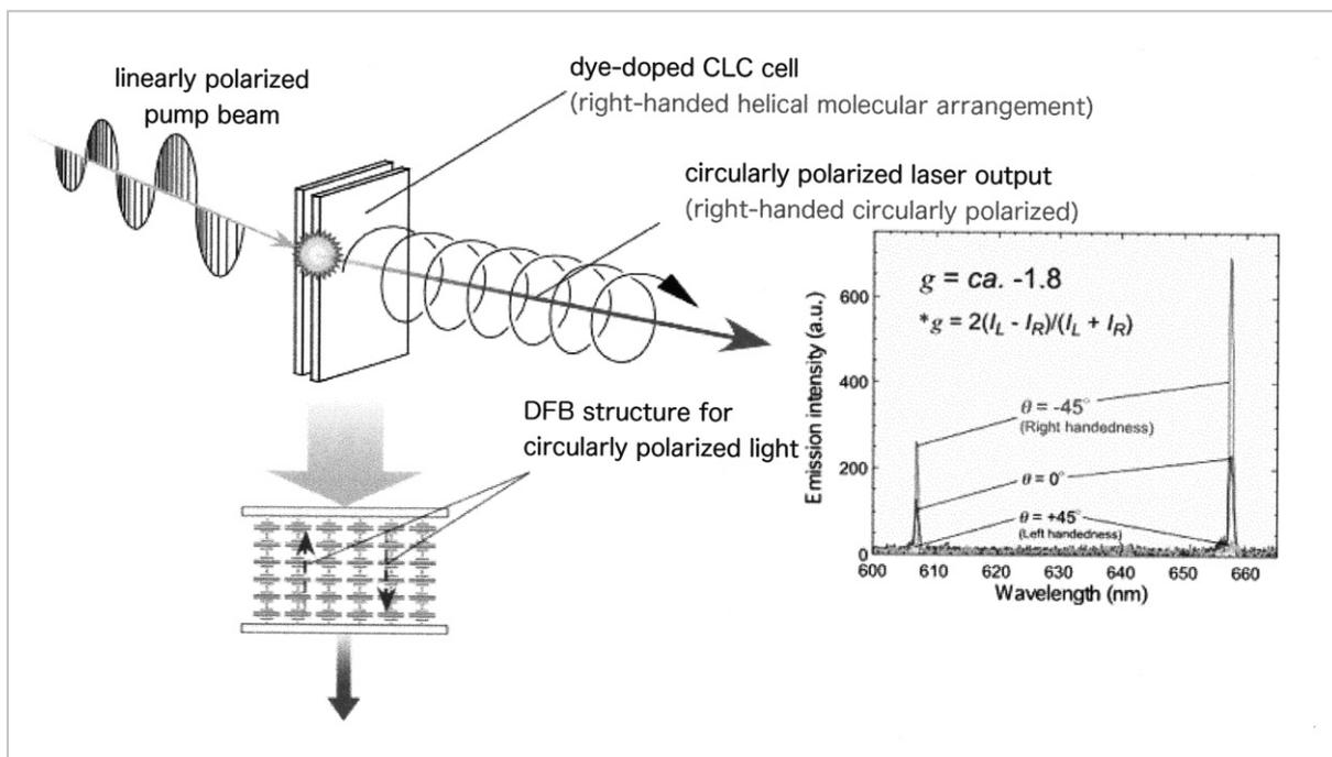
**Fig. 10** Supramolecular helical structure of cholesteric liquid crystals and photonic band-gap laser oscillation
