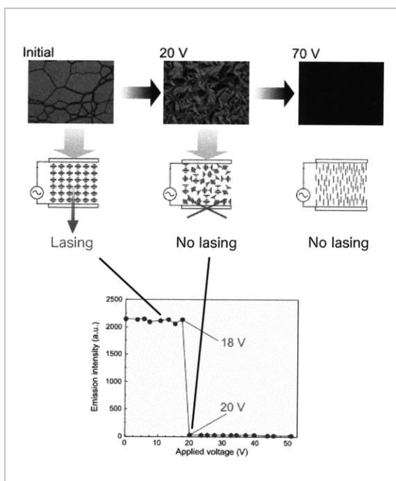
**Fig. 11** Electric field control of photonic band-gap laser oscillation
