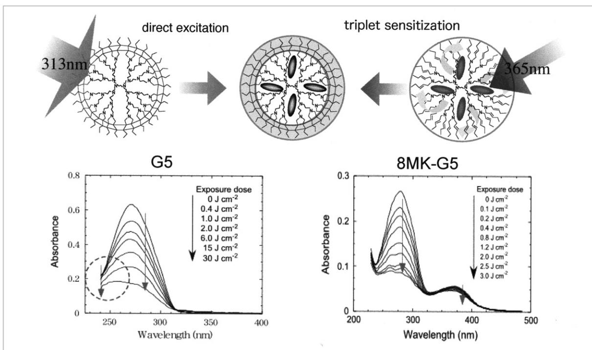
**Fig.9** Triplet-sensitized photochemical reaction of a photocrosslinkable dendrimer
