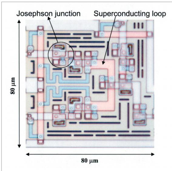
**Fig.5** Microphotograph of an SFQ cell
