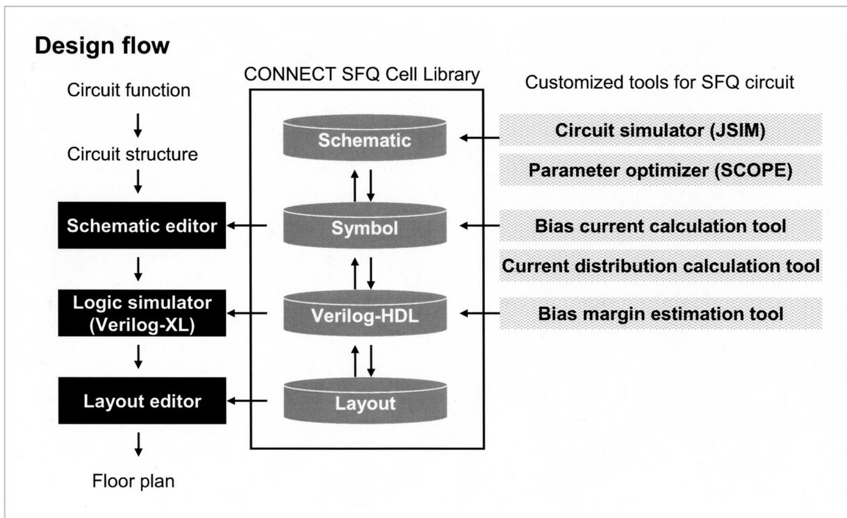
**Fig.4** Design flow of a large-scale SFQ circuit
