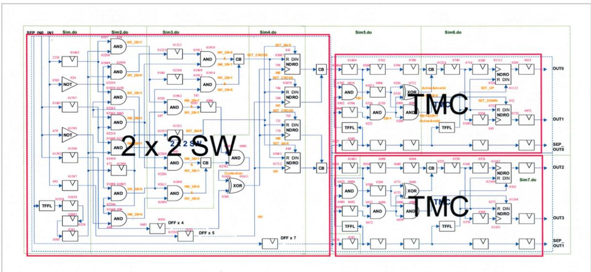
**Fig.7** Block diagram of the network switch circuit
