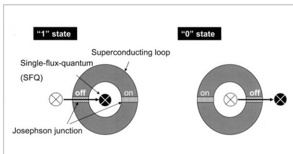
**Fig.1** Operation principle of an SFQ circuit
