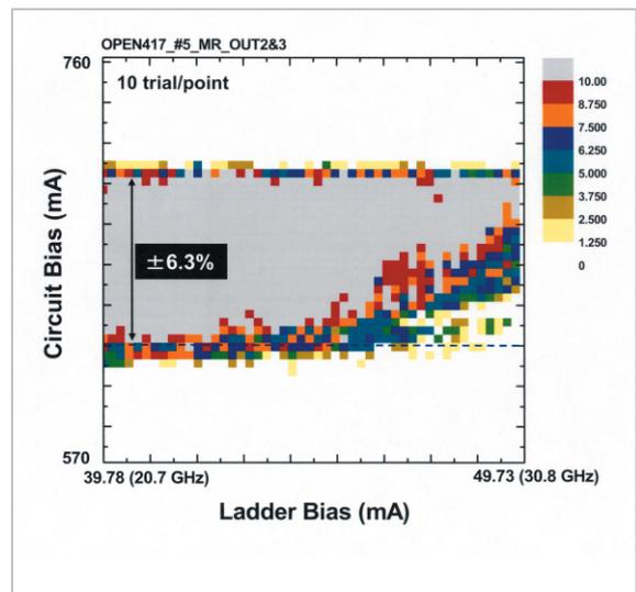
**Fig.8** Operating-speed dependence in the normal range of operation
