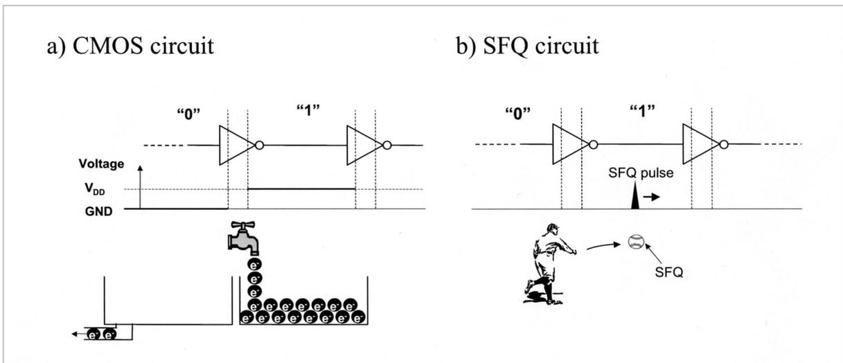
**Fig.3** Comparison of CMOS circuit operation and SFQ circuit operation
