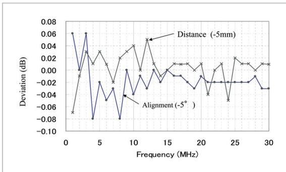
**Fig.5** Effect of loop antenna face-to-face alignment accuracy on propagation characteristic
