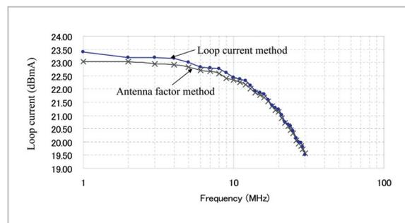
**Fig.7** Frequency characteristic of loop current (standard loop antenna)
