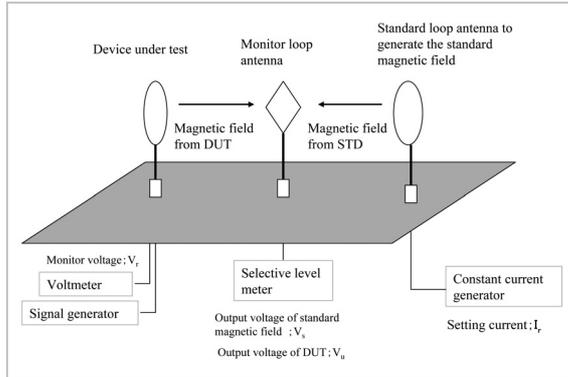
**Fig. 1** Loop antenna calibration using standard magnetic field method (LC method) (For calibration of transmitting loop antenna)
