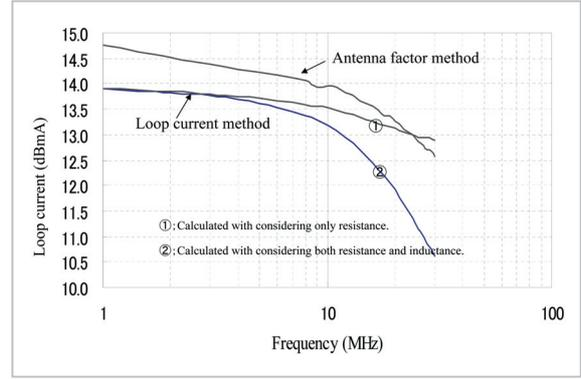
**Fig.8** Frequency characteristic of loop current (general-purpose loop antenna)
