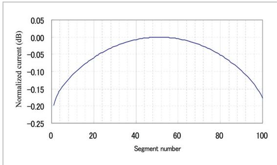
**Fig.4** Transmitting loop current distribution characteristic based on moment method
