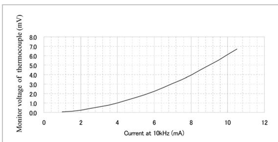
**Fig.3** Relationship between loop antenna input current and monitored voltage
