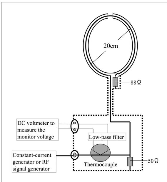
**Fig.2** Example of general-purpose loop antenna setup
