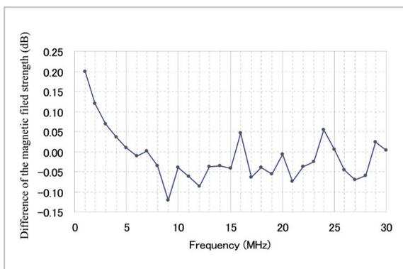
**Fig. 9** Example of difference in magnetic field strengths set by AF method and LC method
