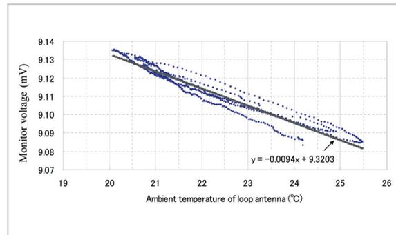
**Fig.6** Temperature characteristic of monitored voltage (general-purpose loop antenna)
