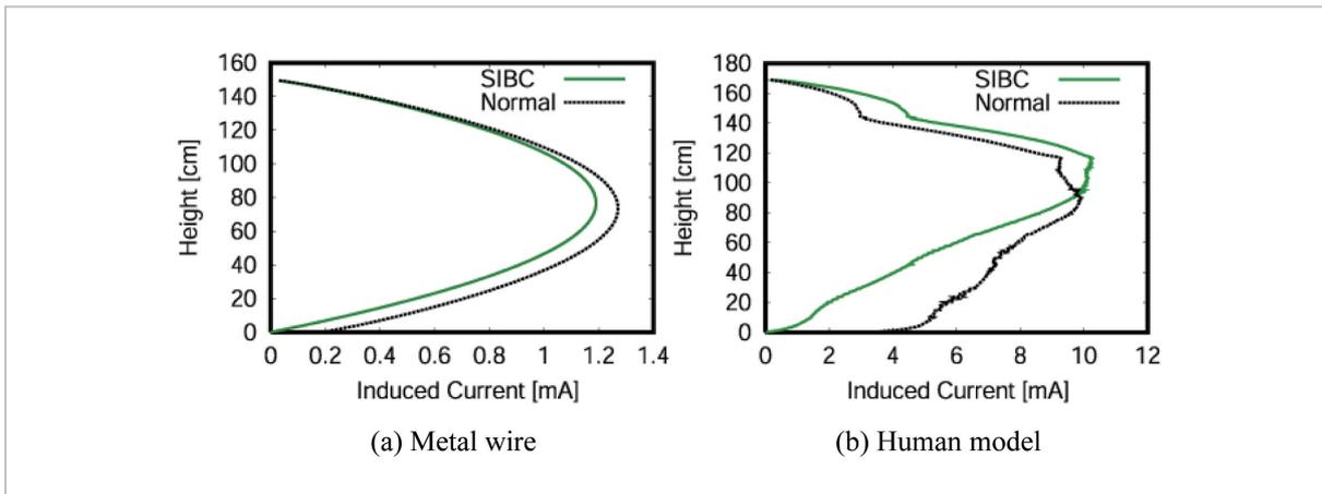
**Fig.5** Induced current distribution on the low-loss ground plane
