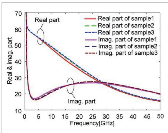
**Fig.7** Results of dielectric constants measurements of blood using the open-ended coaxial probe
