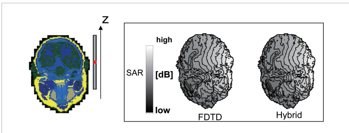
**Fig.4** Results of SAR calculation for the interior of the human head in close proximity to a dipole antenna
