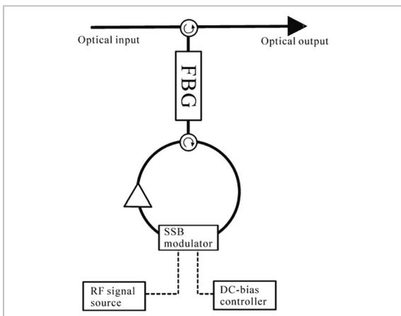
**Fig. 9** Configuration of variable delay
