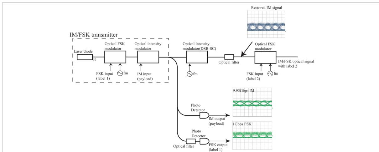
**Fig.6** Optical label transmission based on optical FSK modulation and label swapping
