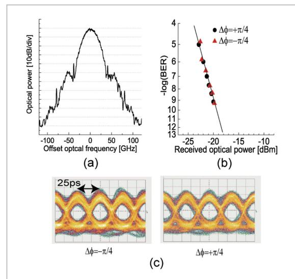
**Fig.8** High-density 80-Gbps transmission based on DQPSK modulation (a) optical spectrum, (b) bit error rate, and (c) demodulated signal waveform
