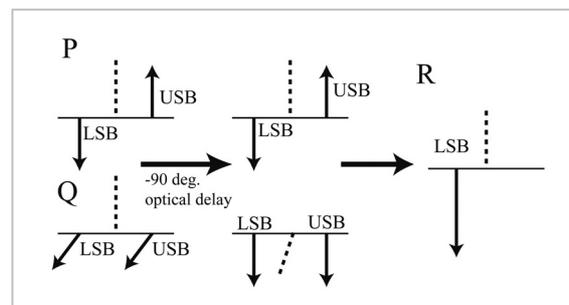
**Fig.4** Operating principle of optical FSK modulator (LSB: generation of components with downward frequency shift)
