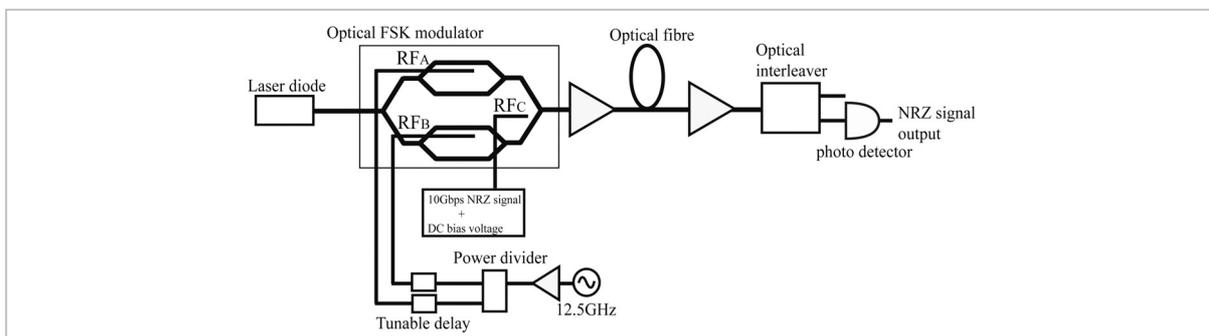
**Fig.5** 10-Gbps FSK transmission experiment
