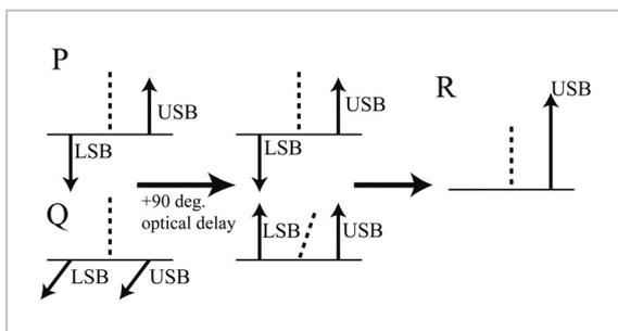
**Fig.3** Operating principle of optical FSK modulator (USB: generation of components with upward frequency shift)
