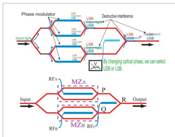
**Fig.2** Optical FSK modulator. Upper figure: schematic diagram. Lower figure: device structure
