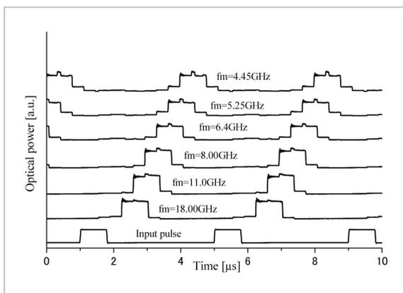
**Fig. 11** Delay controlled optical signal
