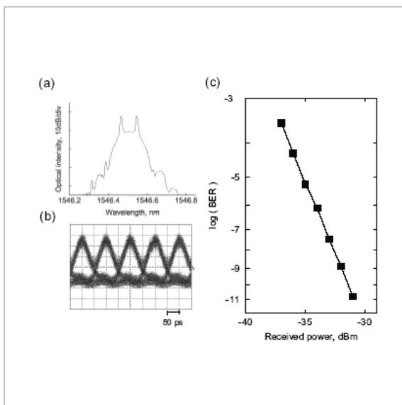
**Fig.7** High-density transmission using optical CPFSK modulation (a) optical spectrum, (b) demodulated signal waveform, and (c) bit error rate
