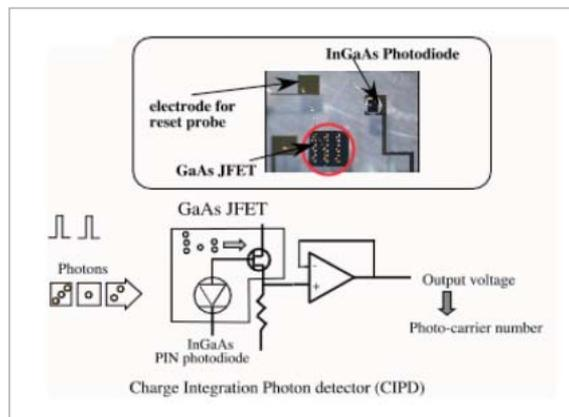
**Fig. 1** Schematic diagram of telecommunications wavelength charge integration photon detector (CIPD)
