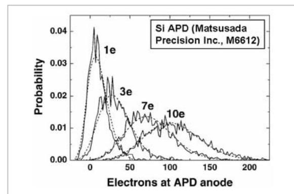
**Fig.6** Rate of electron generation after multiplication with Si APD for visible light with average numbers of generated photo-carriers of 1, 3, 7, and 10
