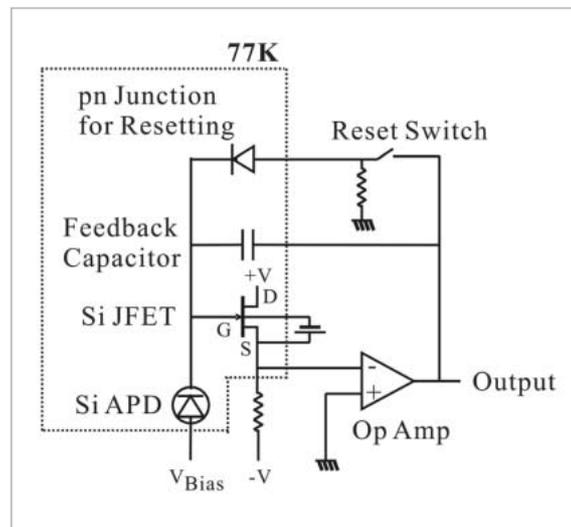
**Fig.4** Schematic diagram of visible and near-infrared CIPD. Operating temperature is 77 K with the exception of the operational amplifier
