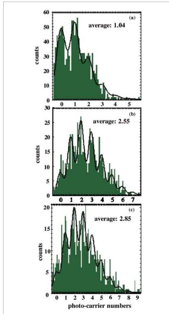
**Fig.2-2** Multipeak structure of photo-carrier distribution
