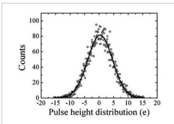
**Fig.5** Charge-converted noise distribution of visible and near-infrared CIPD circuit
