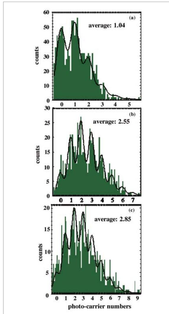
**Fig.2-2** Multipeak structure of photo-carrier distribution
