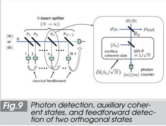
**Fig.9** Photon detection, auxiliary coherent states, and feedforward detection of two orthogonal states
