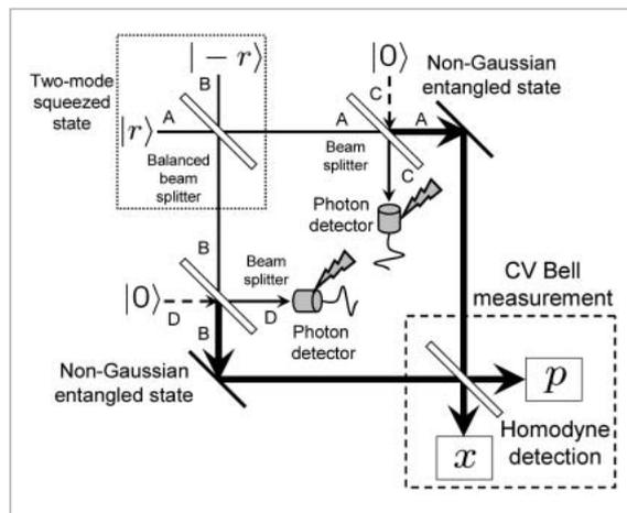
**Fig.3** Non-Gaussian operation on Gaussian entangled states
