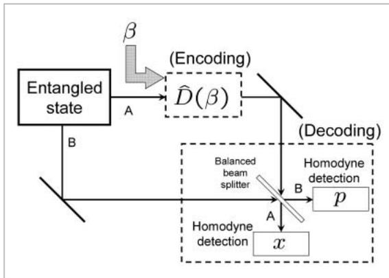
**Fig.5** Schematic diagram of quantum dense coding channel
