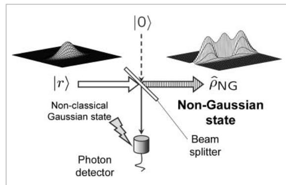
**Fig.2** Schematic diagram of Schrödinger-cat-like state generation scheme based on measurement-induced non-Gaussian operation using beam splitters and photon detectors
