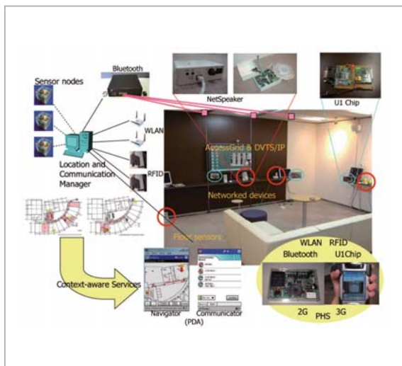
Fig. 8 "Smart space" consisting of various sensors and position estimation systems
