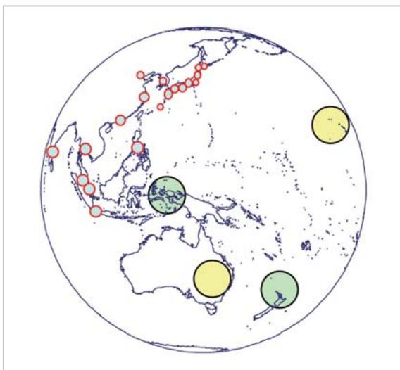
**Fig. 2** Beam direction (MBA beams denoted by small circles, APAA beams denoted by large one)
