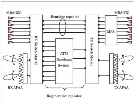
**Fig. 1** Block diagram of the transponder
