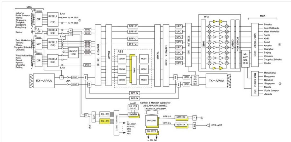
Fig.5 Detailed block diagram of the transponder
