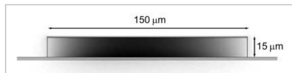
**Fig.4** Electric field distribution of GaSb-based quantum cascade laser fabricated on GaAs substrate based on single plasmon waveguide
