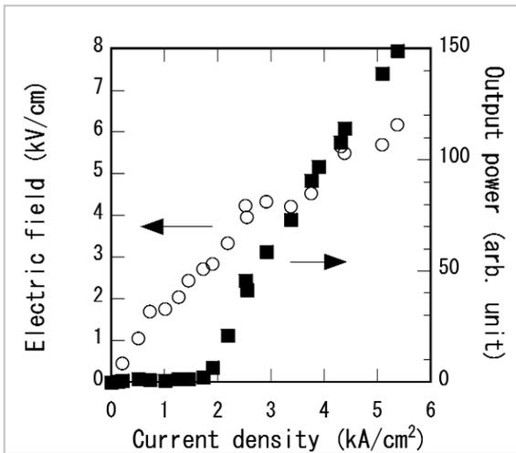
**Fig.5** Electric field vs. current density characteristics and terahertz wave output power vs. current density characteristics for GaSb/AlSb-based quantum cascade laser
