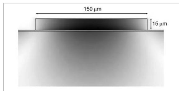
**Fig.3** Electric field distribution of GaSb-based quantum cascade laser fabricated on GaSb substrate based on single plasmon waveguide
