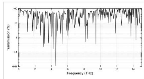
**Fig.4** Transmission spectrum of air with light path of approximately 80 cm
