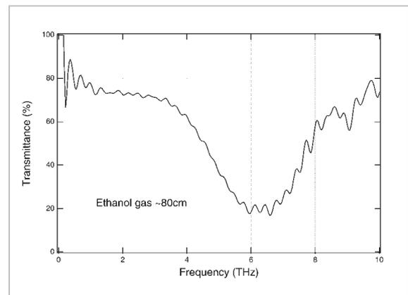
**Fig.5** Transmission spectrum of ethanol gas with light path of approximately 80 cm
