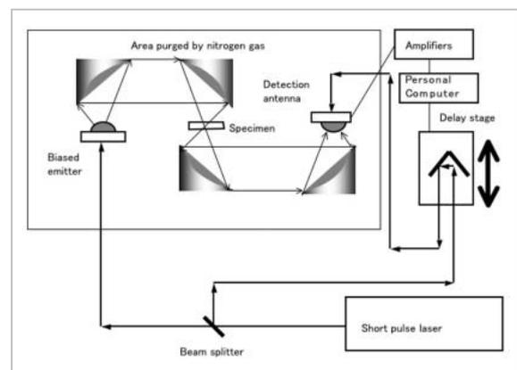
**Fig. 1** Schematic drawing of typical THz-TDS system
