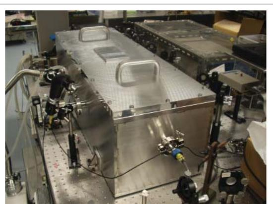
**Fig.3** Outward appearance of broadband THz-TDS system
