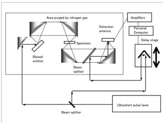
**Fig.2** Schematic drawing of broadband THz-TDS system
